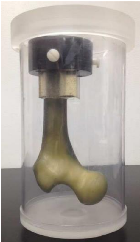
Figure 1. Clear representation of proximal femur fixture/humidity chamber. Our current fixture is opaque.
